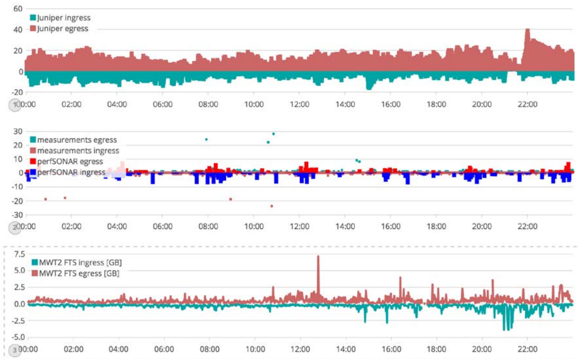
Figure 16: A timelion visualization showing combined information from three different sources. Top: bandwidth seen by the sites border switch. Middle: bandwidth measurements reported by perfSONAR. Bottom: File Transfer Service (FTS) utilization.
