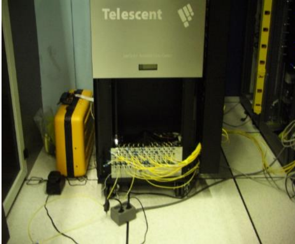
Figure 109: The Telescent optical switch was integrated into a test environment in the US LHCNet infrastructure at CERN.
