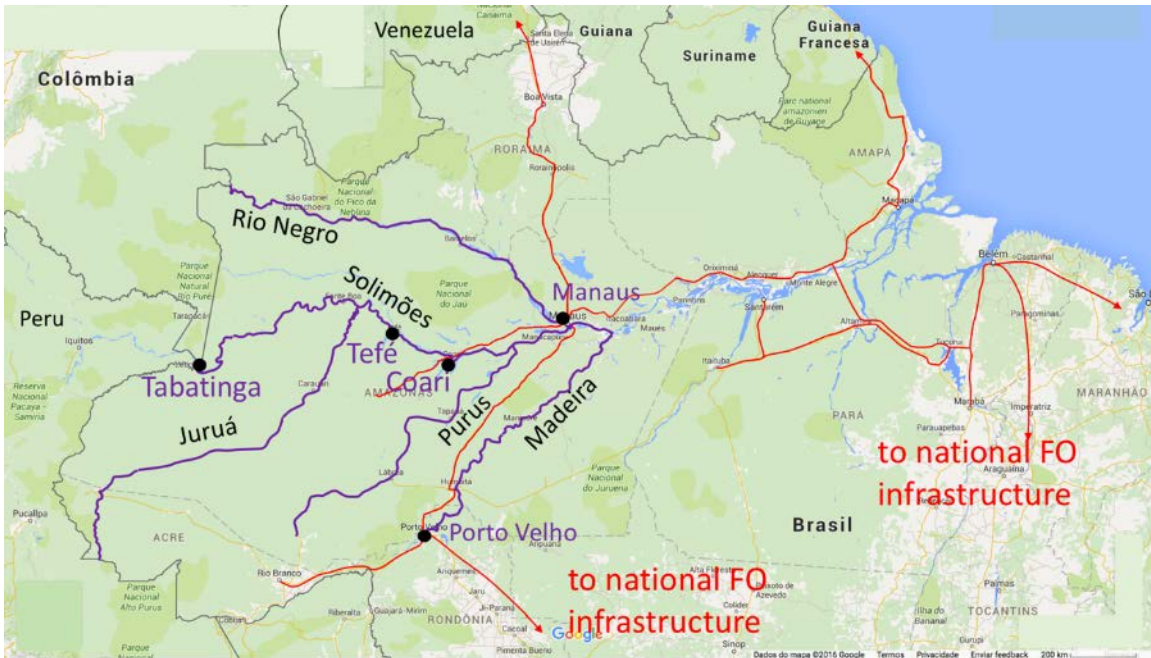
Figure 72: Proposed Infovias (data highways) of the Amazonia Connected programme (red lines indicate existing fiber; blue lines are proposed sub-fluvial fiber)
