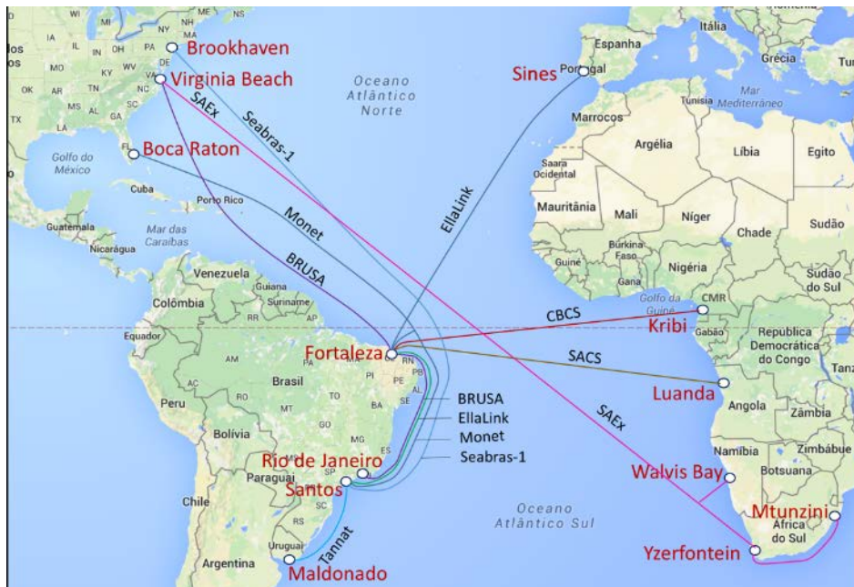
Figure 76: Expected new cables in the South Atlantic, showing topology and landing points (CMR = Cameroon)
